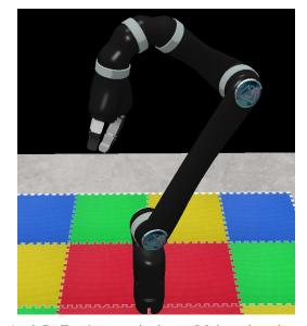
Fig. 1: 6 DoF robot manipulator (Mujoco based model), where we incorporate a large number of safety constraints (>100). We propose a QP based model-free control framework with guaranteed feasibility and continuity properties.
